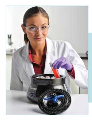
Rotor selection is critical when it comes to sample safety and centrifuge performance. Thermo Scientific™ Fiberlite™ carbon fiber rotors are designed to deliver exceptional performance without fatigue or corrosion for worry-free operation spin after spin.
